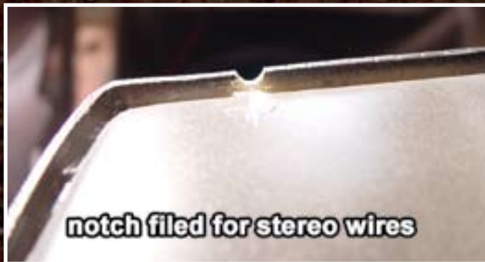
installing stereo housing
